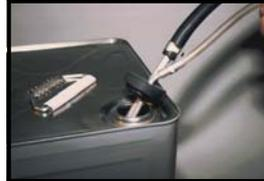
The fluid can cap can be inserted into an 18-liter can or a pail can, to protect the fluid against moisture.
