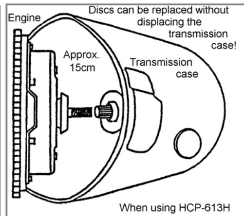
\* If only a 15cm opening is available, as shown in the figure, the transmission does not need to be displaced in order to carry out the work. (for Altos, etc.)
