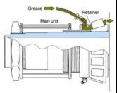
\* The main unit is rotated to close the gap between the main unit and the retainer.
