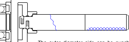
How oil seals are punched
